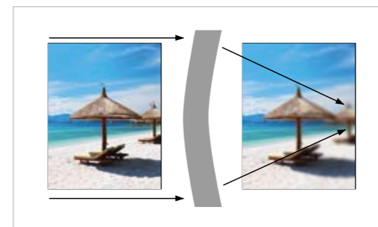
Vacuum-forming produces a lens of uniform thickness which distorts vision.
